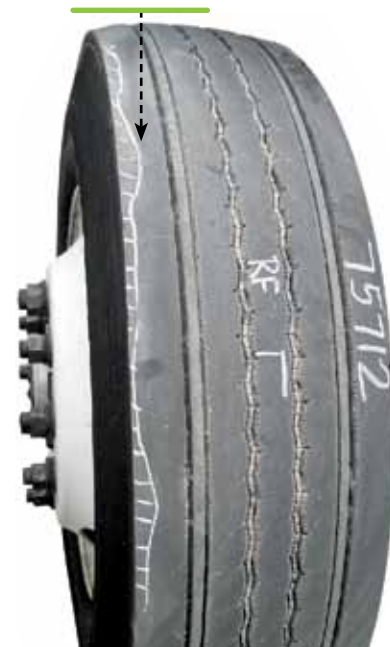
Shoulder wear has spread across to the main ribs.
